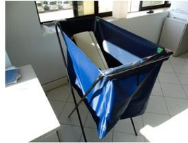
4. Wrap the unit with the wall bag. Pay attention to the direction of the bag: the straps must be forward and the water drain downward. Tighten the strings of the bag to make it well adhere to the unit. The bag will tighten between the wall and the unit.
